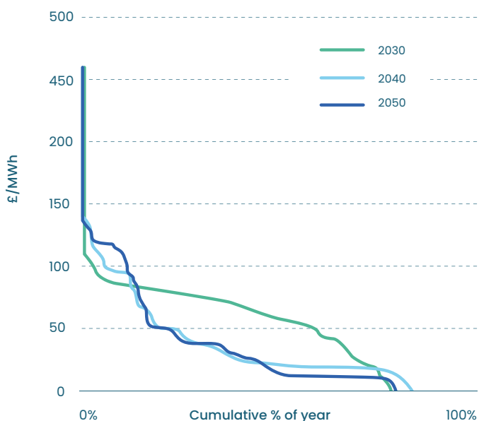
Figure 2. Wholesale electricity prices could be lower for longer in an integrated energy system (Source: “Developing a Whole Systems Approach to Explore Pathways to Net Zero”, Centrica, FTI)
